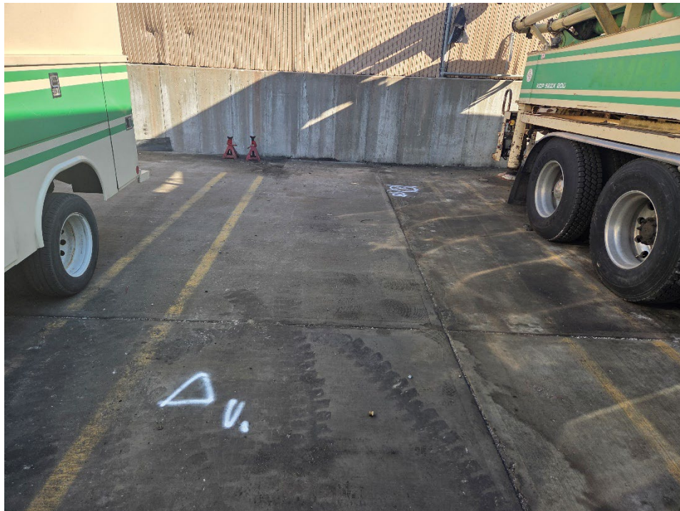
Photo 4. Proposed vapor and boring locations.
