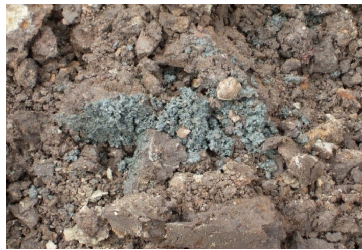
Photo 14: Grayish-stained soil with high PID readings from Area 5.
