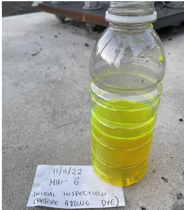
Photograph 1: 11/11/2022 groundwater dye test before dye was introduced to MW-6 (onsite well)
