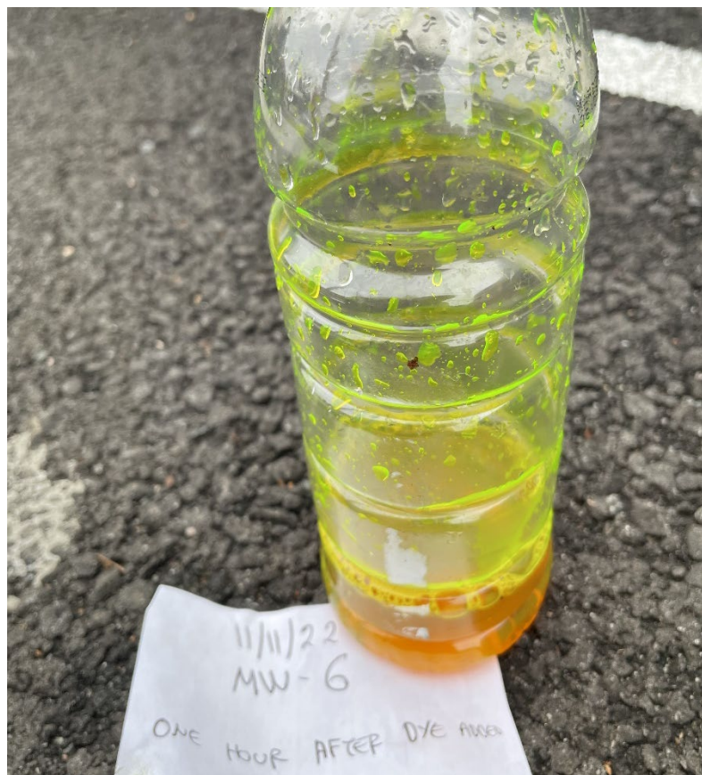
Photograph 2: 11/11/2022 groundwater dye test after dye was introduced to MW-6 (onsite well)
