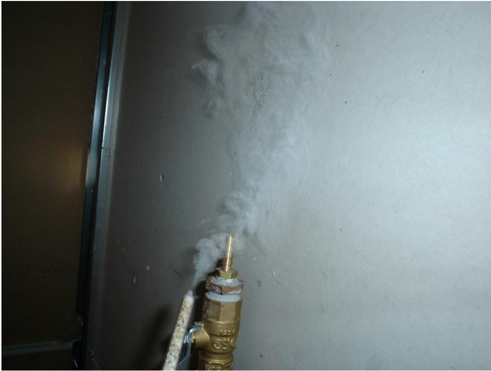
Photo 51 — Smoke test at sample port (July 7, 2006)
