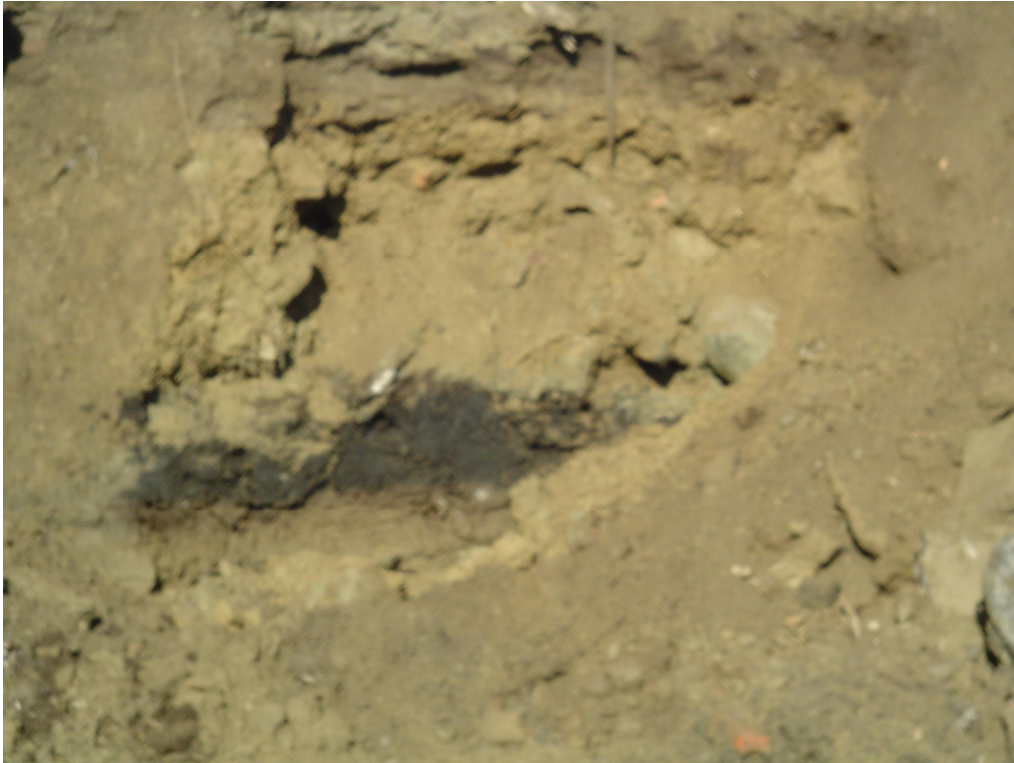
Photo 9 — View of oil sludge layer exposed in the southern landfill area ( February 23, 2005)
