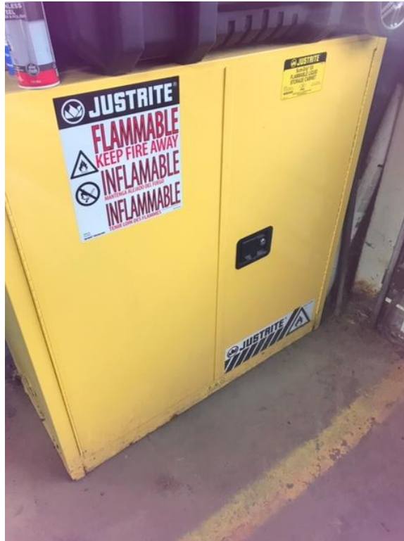
Photo 27: Locked Flammable Liquid Cabinet
