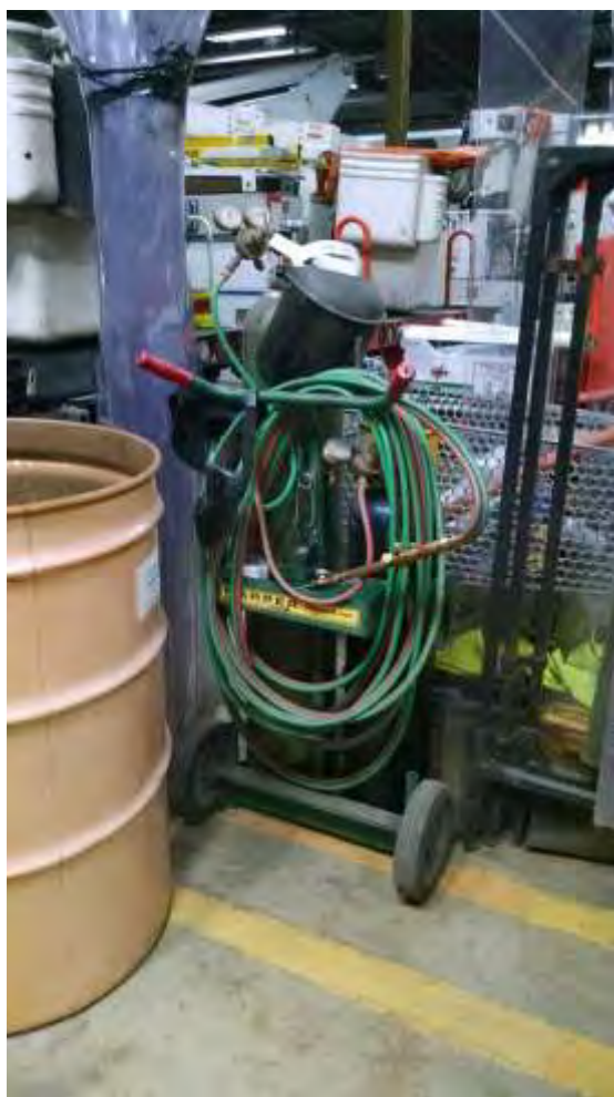
Photo 39: Acetylene Dissolved Gas Cylinder
