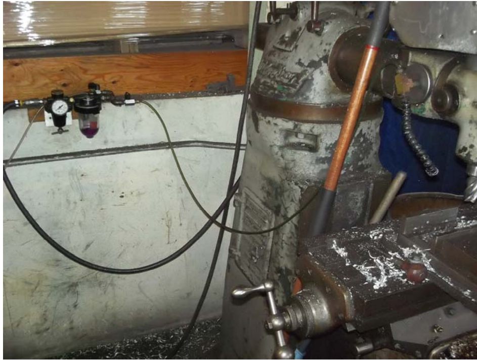
View of drill with lubrication system.
