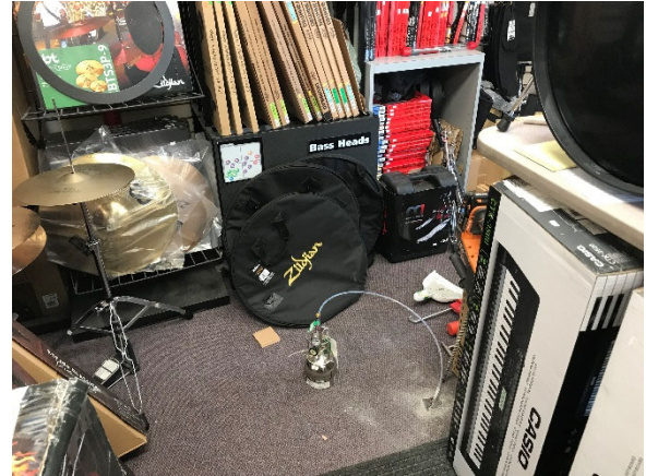
#8: VIEW OF SUB-SLAB SOIL GAS SAMPLE SS-4
