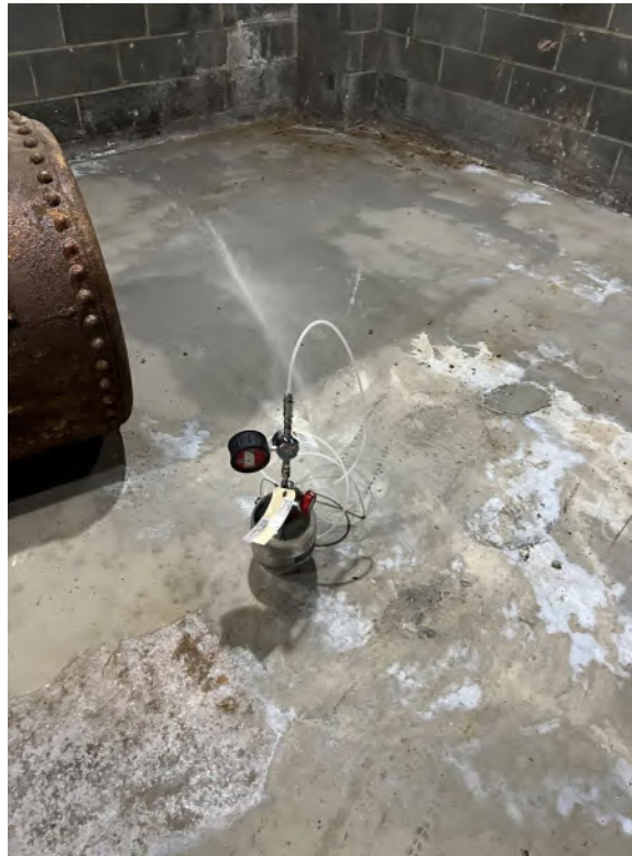
Photograph 10 – Sub-slab vapor sample collection.
