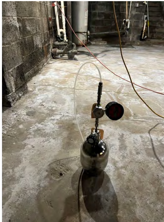
Photograph 11 – Sub-slab soil vapor sample collection.
