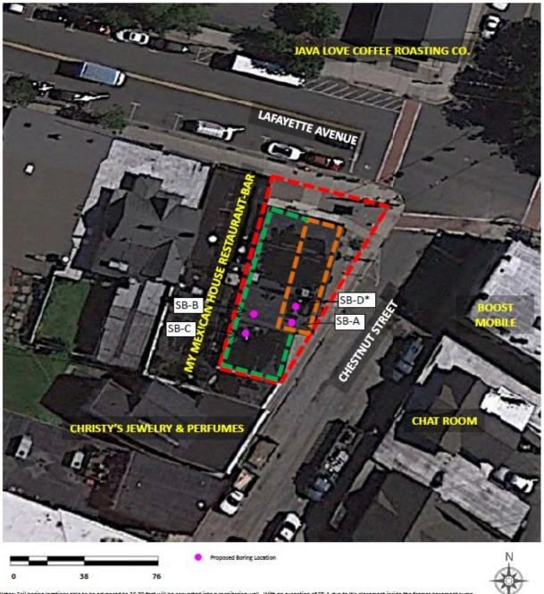
Notes: Soil boring locations able to be advanced to 26-30 feet will be converted into a monitoring well. With an exception of SB-A due to It's placement inside the former basement Boring Locations: SB-B inside basement sump SB-B inside former boiler room closest to former dry-cleaning equipment SB-C Located under the former dry cleaning machine. SB-D placed adjacent the boring with the most field evidence of impacts it's placement will be determined in the field.
