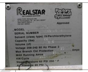
Plate on the back of the dry cleaning machine in the Touch of Class Cleaners unit.
