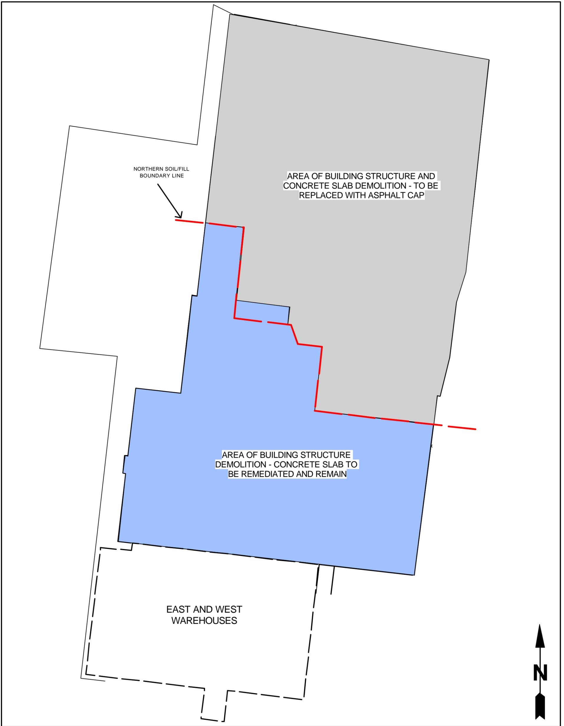
AREA OF BUILDING STRUCTURE AND CONCRETE SLAB DEMOLITION - TO BE REPLACED WITH ASPHALT CAP
