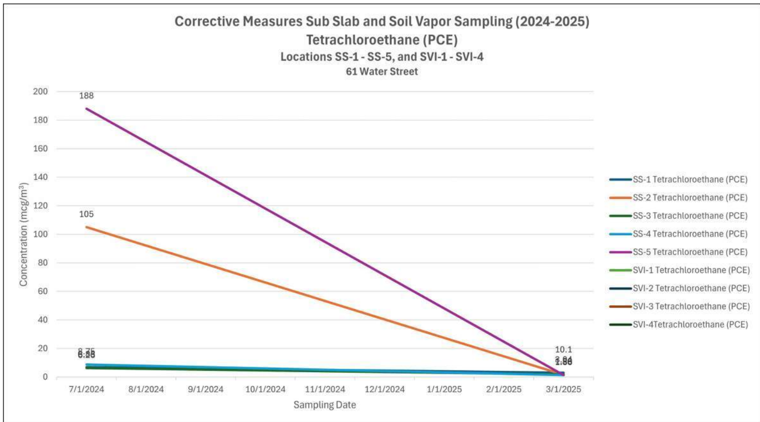
Corrective Measures Sub Slab and Soil Vapor Sampling PCE (2024-2025)
