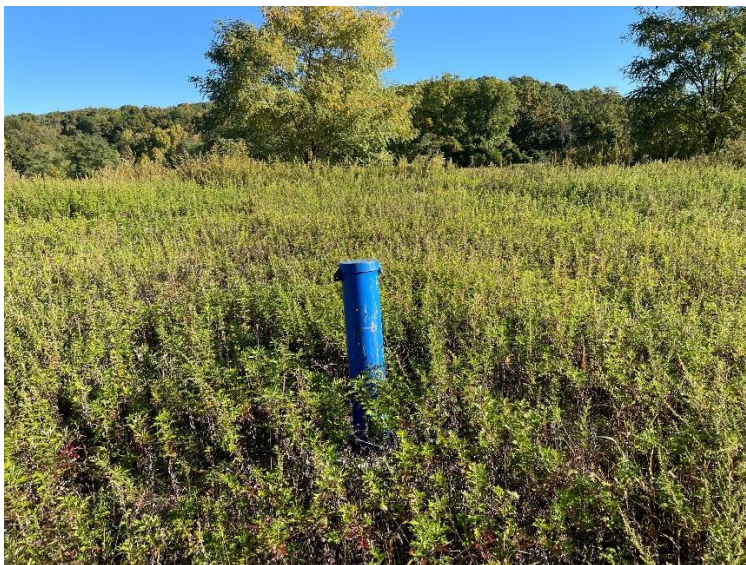
Photo 6 Piezometer installed by others during geotechnical investigation. Needs lock on cover.
