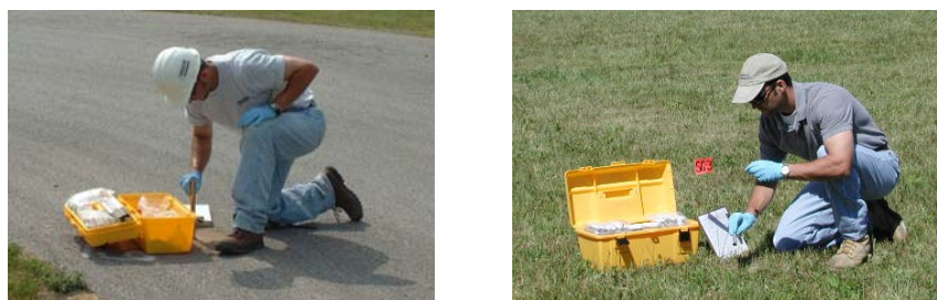
Figure 1 — Installation of Samplers with BESURE Sample Collection Kit™
