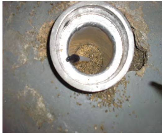
Installed permanent vapor point with gravel pack
