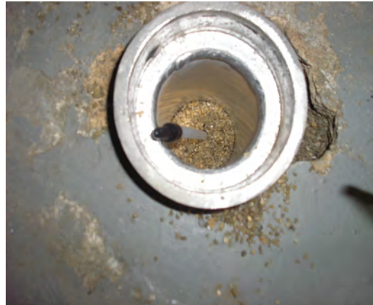
Installed permanent vapor point with gravel pack
