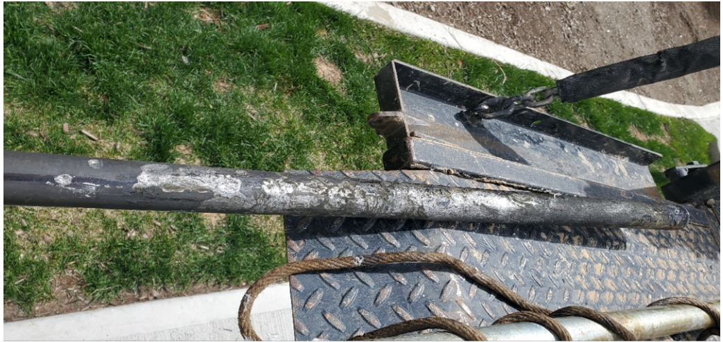
Photograph 3 - Photograph of corrosion on NW-5 internal pipe.
