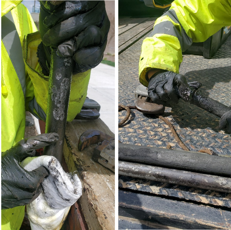
Photograph 1 - Photographs of corrosion on 1-inch internal pipe of NW- 5.
