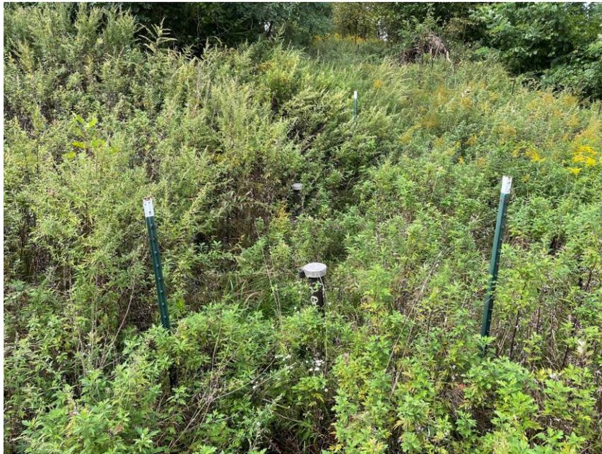
*Photo 5 Typical Site groundwater monitoring wells.*
