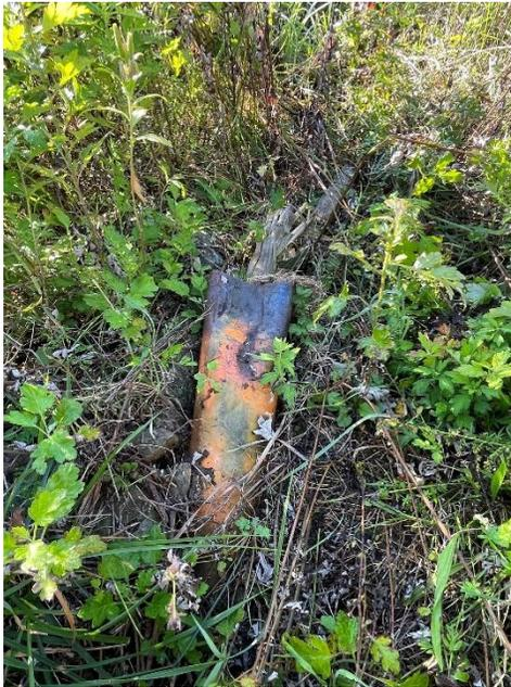
*Photo 3 Damaged Site groundwater monitoring well MW-1 from unknown event – to be decommissioned.*
