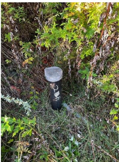
*Photo 2 Typical Site groundwater monitoring wells.*
