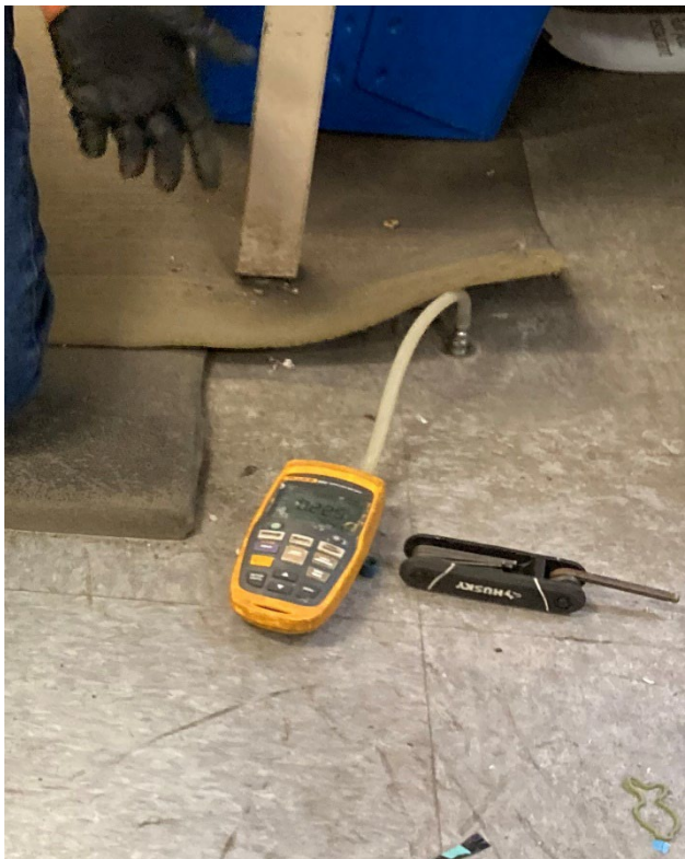
Photograph 14: Vacuum Reading at monitoring point MP-12 inside post office
