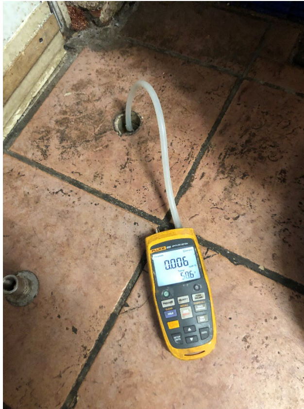
Photograph 11: Vacuum Reading at monitoring point MP-8R inside pizzeria
