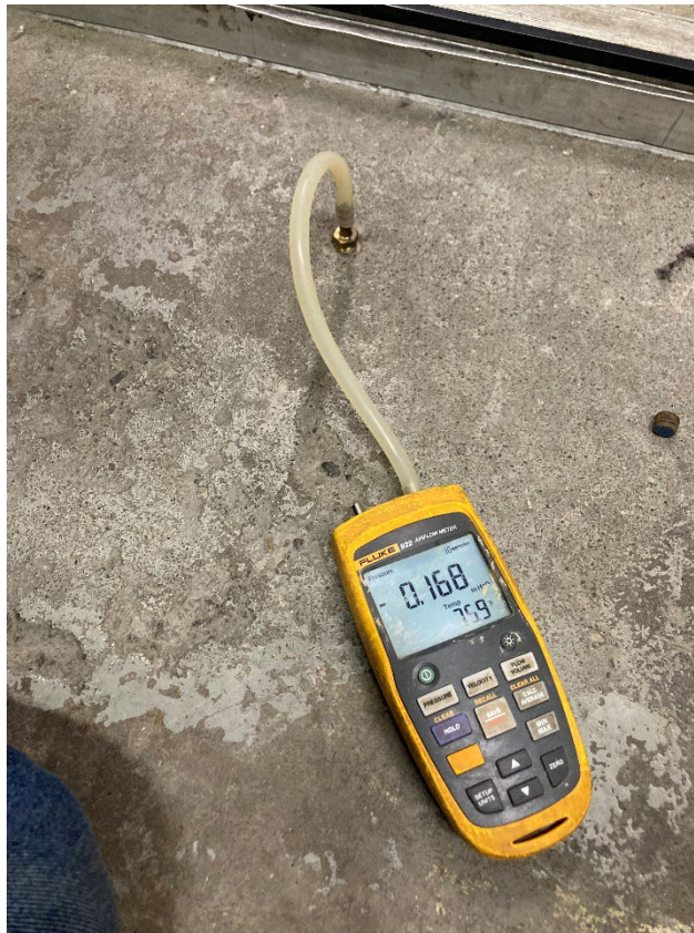
Photograph 9: Vacuum Reading at monitoring point MP-6 inside dry cleaner
