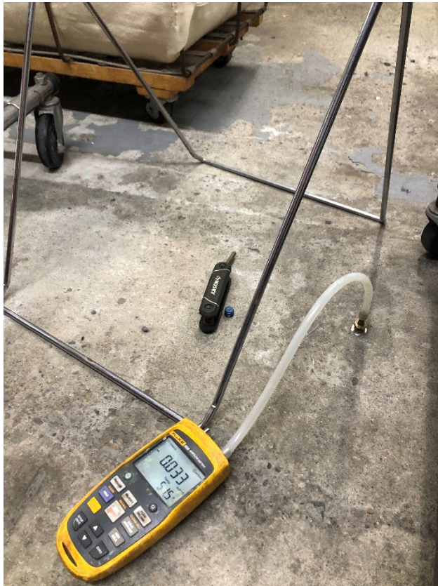
Photograph 8: Vacuum Reading at monitoring point MP-5 inside dry cleaner
