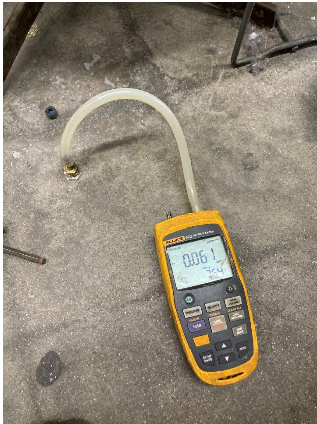
Photograph 10: Vacuum Reading at monitoring point MP-7 inside dry cleaner
