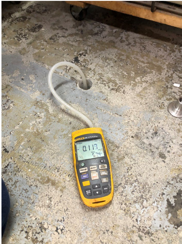
Photograph 30: [2/24/23] Vacuum Reading at monitoring point MP-15 inside dry cleaner
