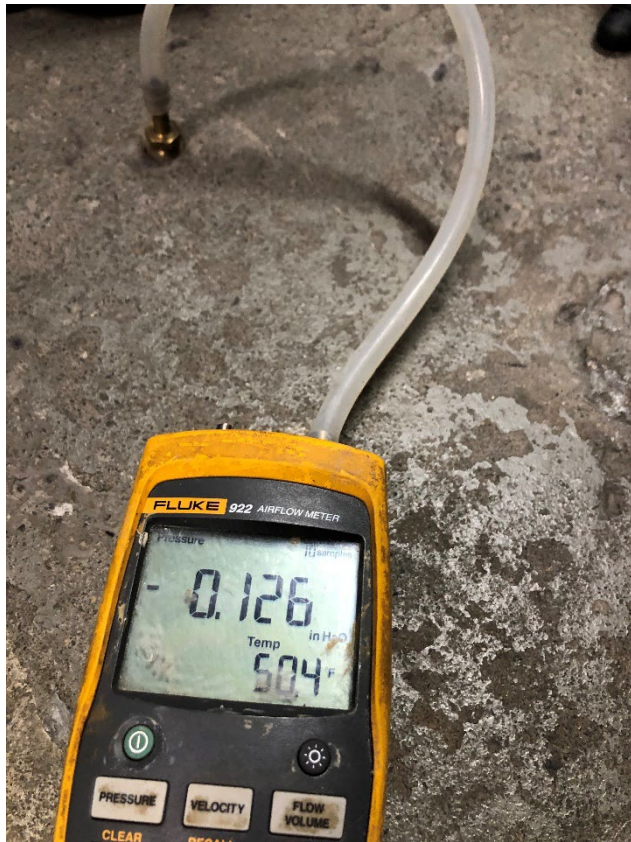
Photograph 27: [2/24/23] Vacuum Reading at monitoring point MP-6 inside dry cleaner
