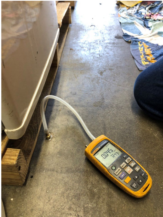
Photograph 28: [2/24/23] Vacuum Reading at monitoring point MP-7 inside dry cleaner
