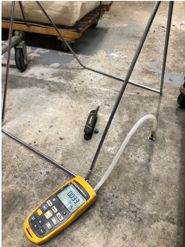
Photograph 26: [2/24/23] Vacuum Reading at monitoring point MP-5 inside dry cleaner
