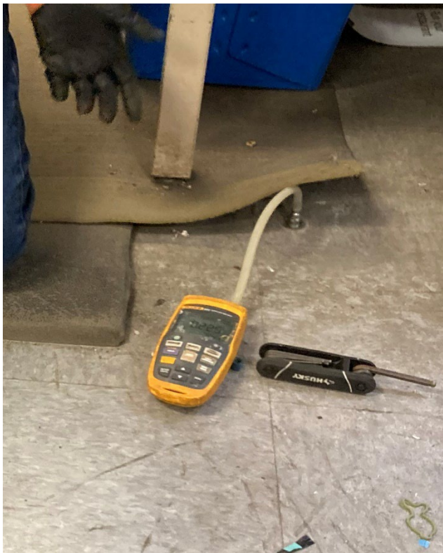
Photograph 14: [5/13/22] Vacuum Reading at monitoring point MP-12 inside post office
