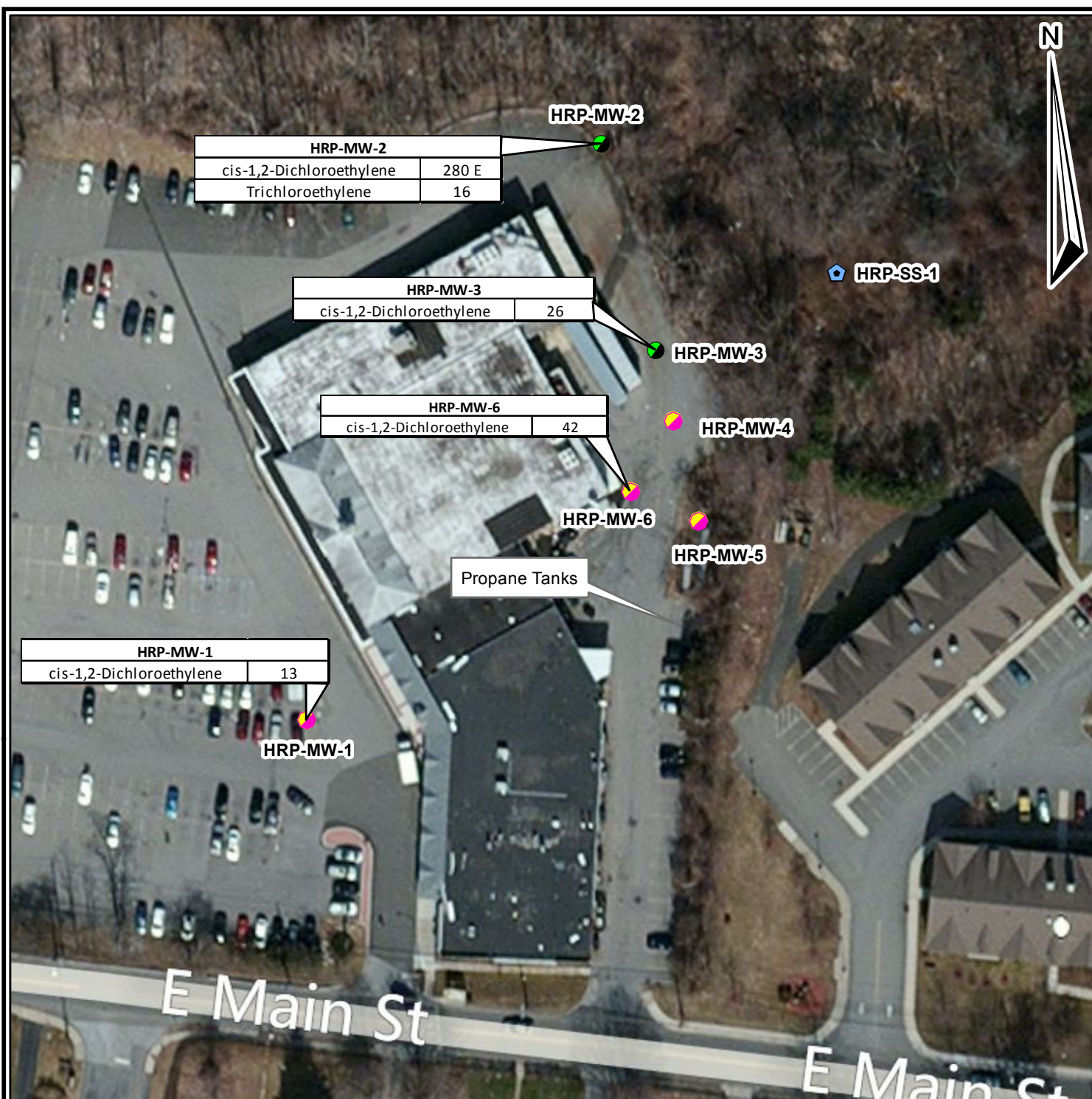
Figure 8 Groundwater VOC Exceedances July 12, 2012 Mr. Cleaners 1360 East Main Street Shrub Oak, Yorktown, New York (Site Code #360117) WA # D006130-27) HRP # NEW9629.P2 Scale 1" = 100'
