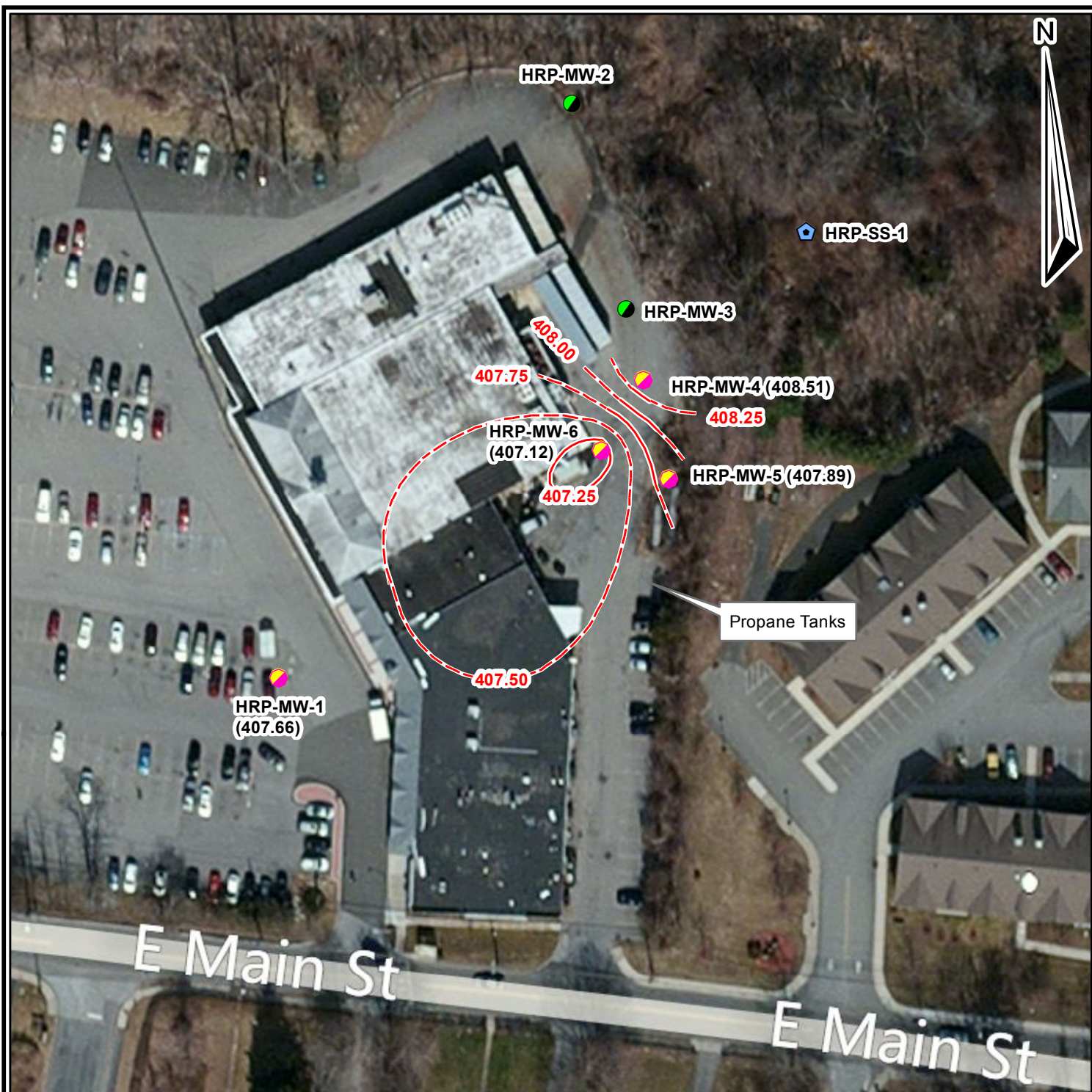
Figure 7B Shallow Groundwater Contours July 12, 2012 Mr. Cleaners 1360 East Main Street Shrub Oak, Yorktown, New York (Site Code #360117) WA # D006130-27) HRP # NEW9629.P2 Scale 1" = 100'
