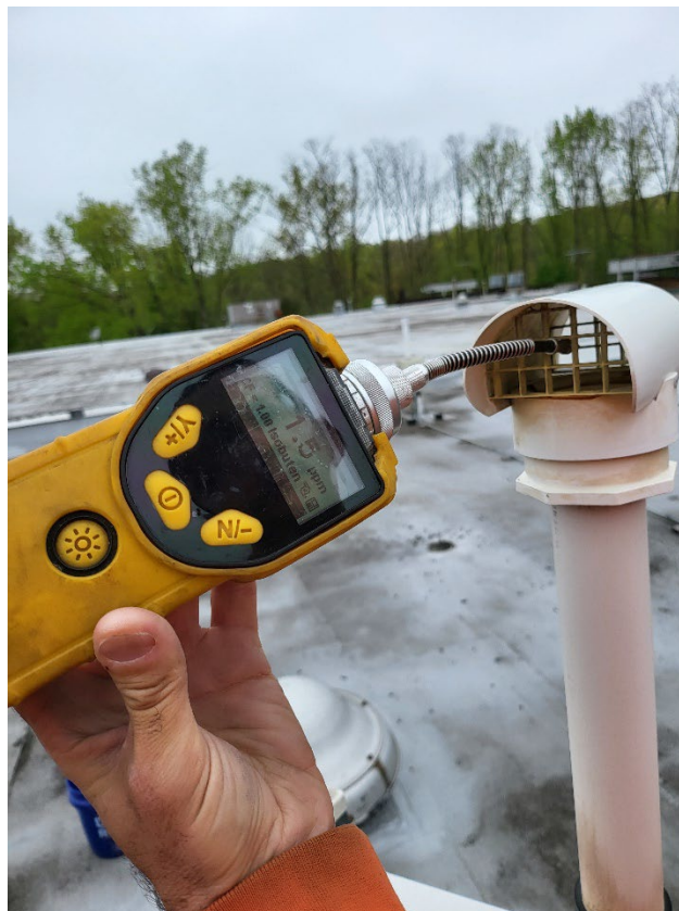
Photograph 18: [5/13/22] Maximum PID reading recorded at discharge stack
