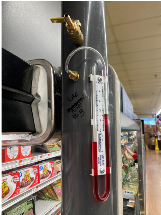
Photograph 10: [5/13/22] Vacuum Reading at extraction point VMP-3
