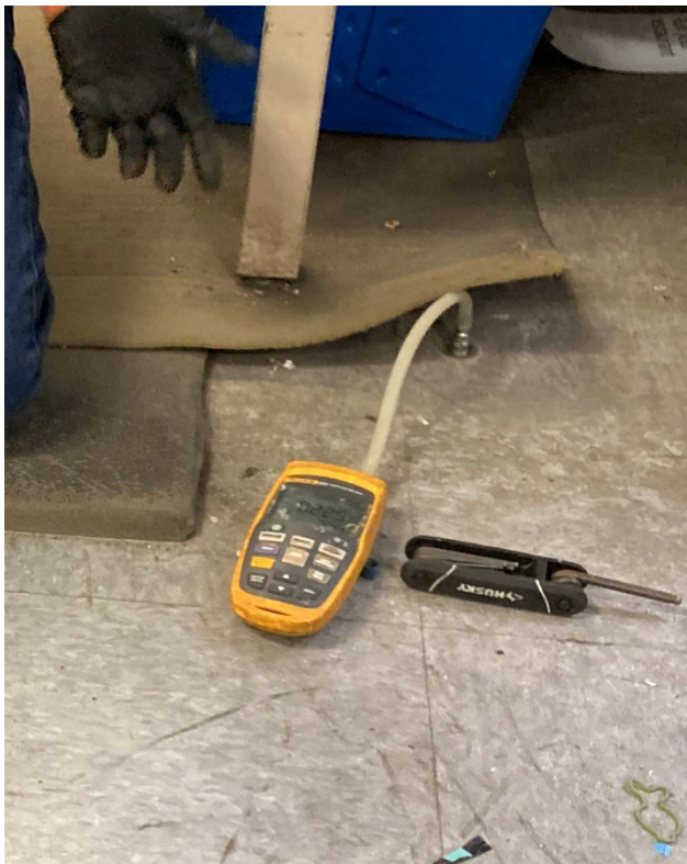
Photograph 14: [5/13/22] Vacuum Reading at monitoring point MP-12 inside post office
