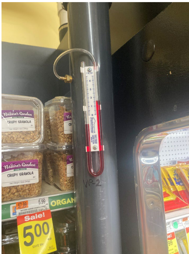
Photograph 8: [5/13/22] Vacuum Reading at extraction point VMP-2
