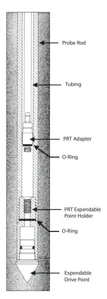
A cross section of probe rods driven to depth and then retracted to allow for soil gas sampling. The PRT adapter and tubing are now fed through the rods and rotated to form a vacuumtight connection at the point holder. The result is a continuous run of tubing from the sample level to the surface.
