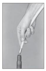
Figure 2. Insertion of tubing and PRT adapter.
