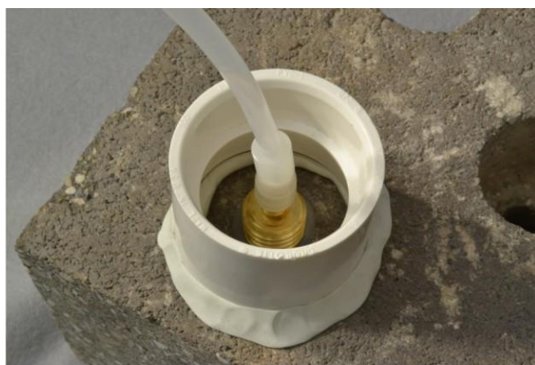
Figure 6. Water dam used for leak detection
