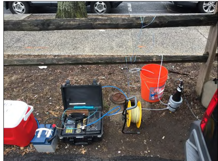
Photograph 8: Low-flow groundwater sampling equipment set up at MW-5.
