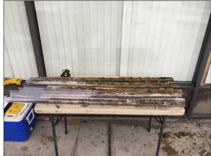
Photograph 2: Soil cores from soil boring SB-10 staged for field screening and sample collection.
