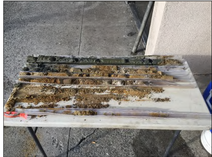
Photograph 6: Soil cores from soil boring SB-15 staged for field screening and sample collection.
