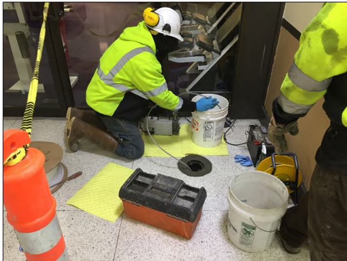
Photograph 7: Development of MW-15.
