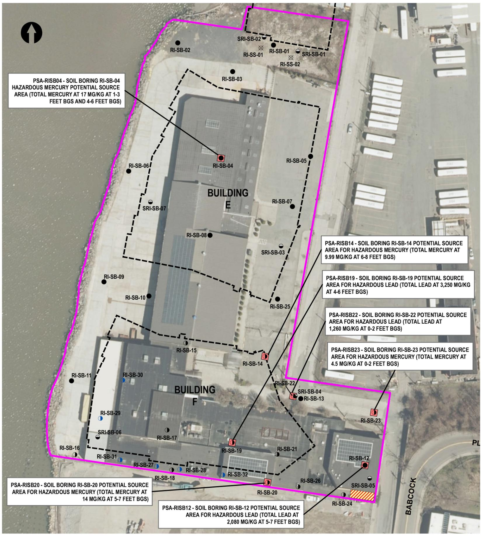
PSA-RISB04 - SOIL BORING RI-SB-04 HAZARDOUS MERCURY POTENTIAL SOURCE AREA (TOTAL MERCURY AT 17 MG/KG AT 1-3 FEET BGS AND 4-6 FEET BGS)
