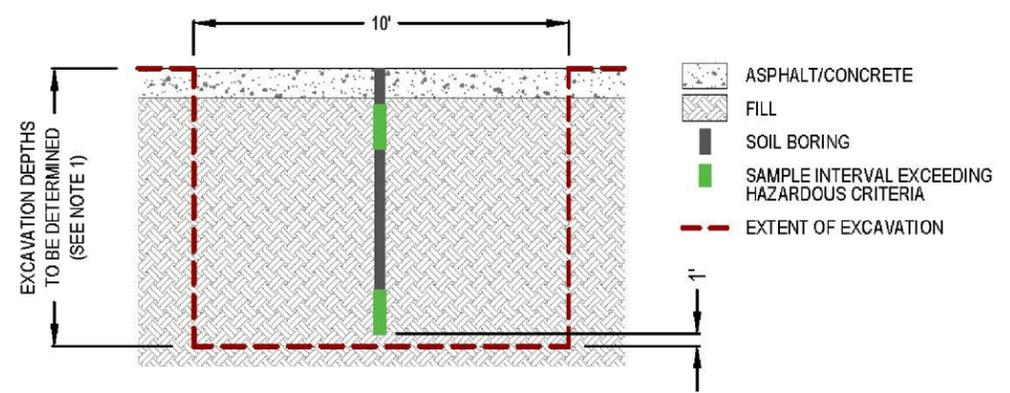
DETAIL 1 - TYPICAL HAZARDOUS METALS PSA EXCAVATION
