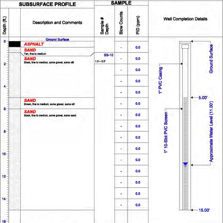
Completion Notes: EOB @ 15' BGS. Hole filled with soil cuttings and bentonite.
