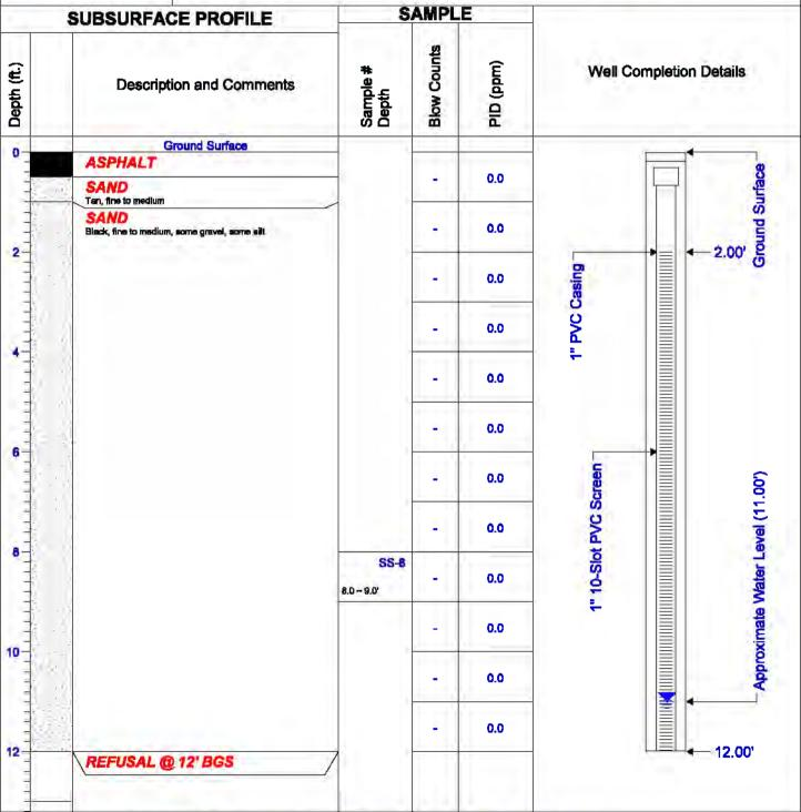
Completion Notes: EOB @ 12' BGS. Hole filled with soil cuttings and bentonite.
