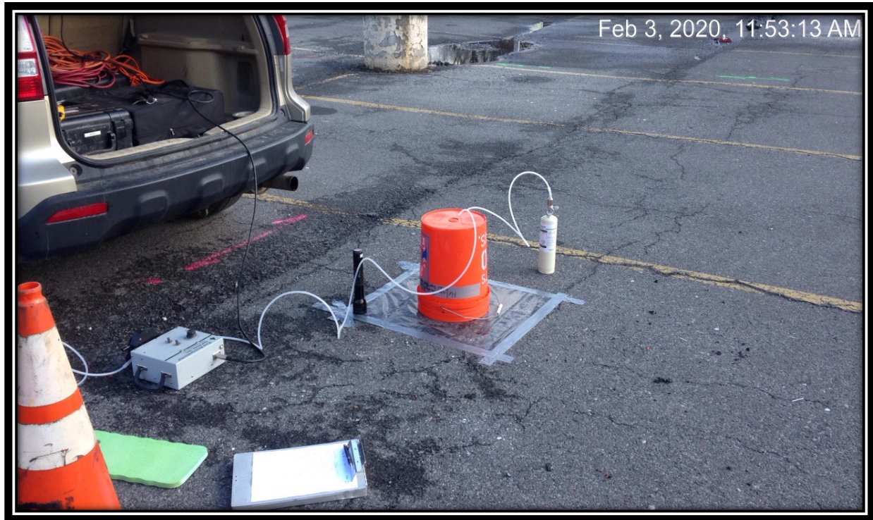
Photograph of soil vapor testing on-site (vapor tightness testing)
