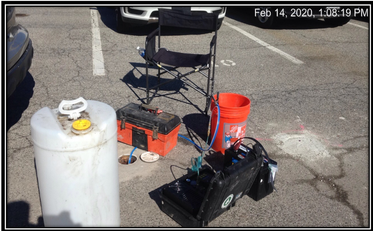
Photograph of monitor well development and low-flow sampling activities
