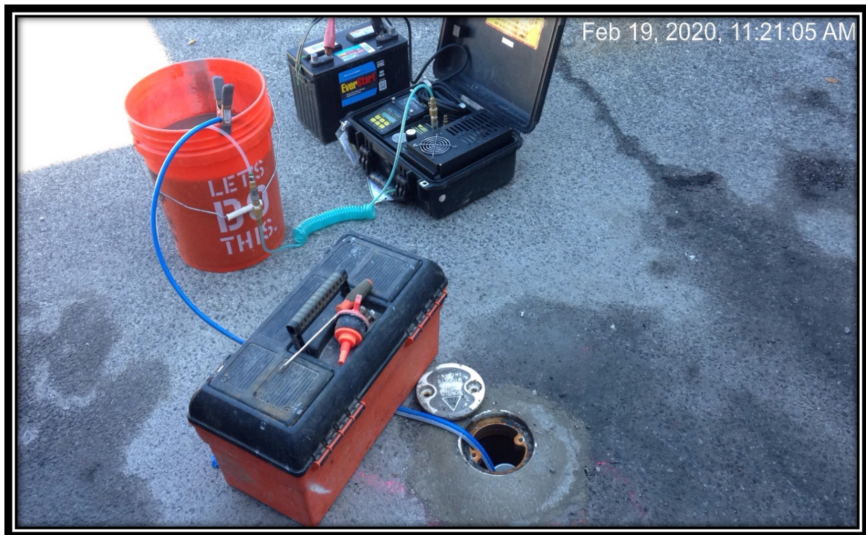
Photograph of development and low flow sampling of a monitoring well on site
