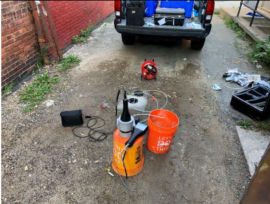
Photo 1: Photograph of low flow sampling at MW-4.
