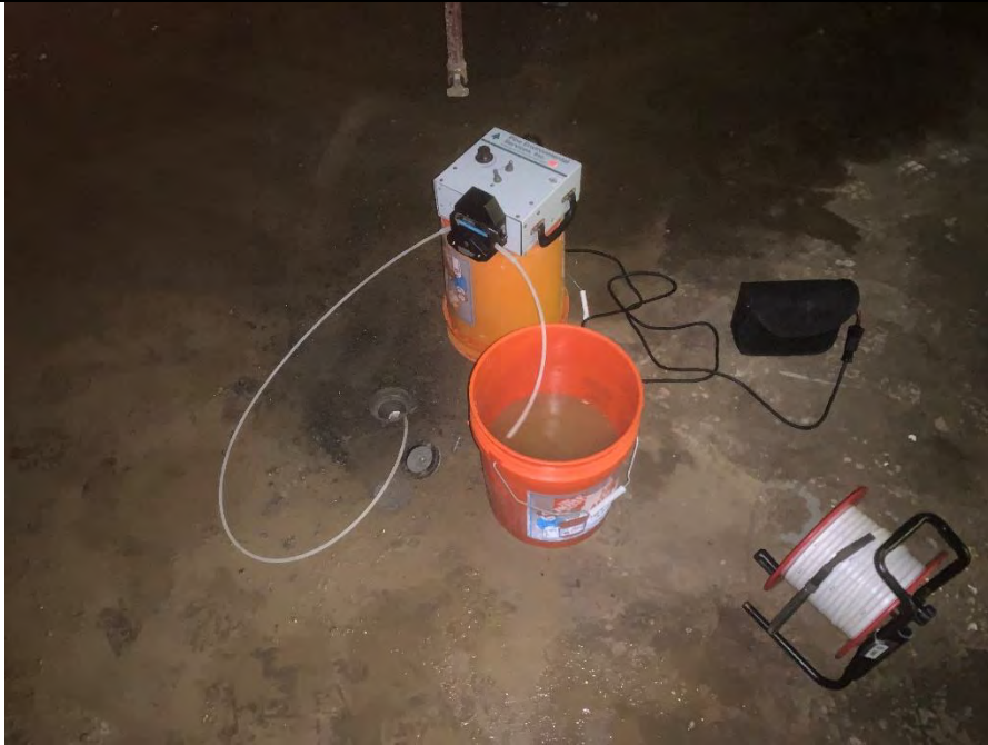
Photo 3: Photograph of well developing at MW-7.
