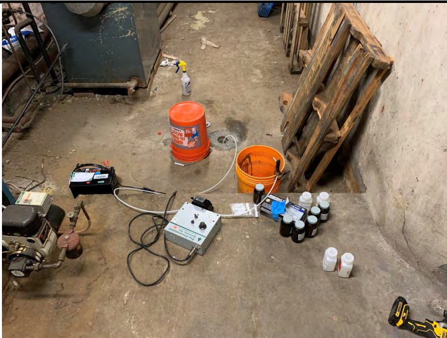
Photo 2: Photograph of low flow sampling at MW-3.
