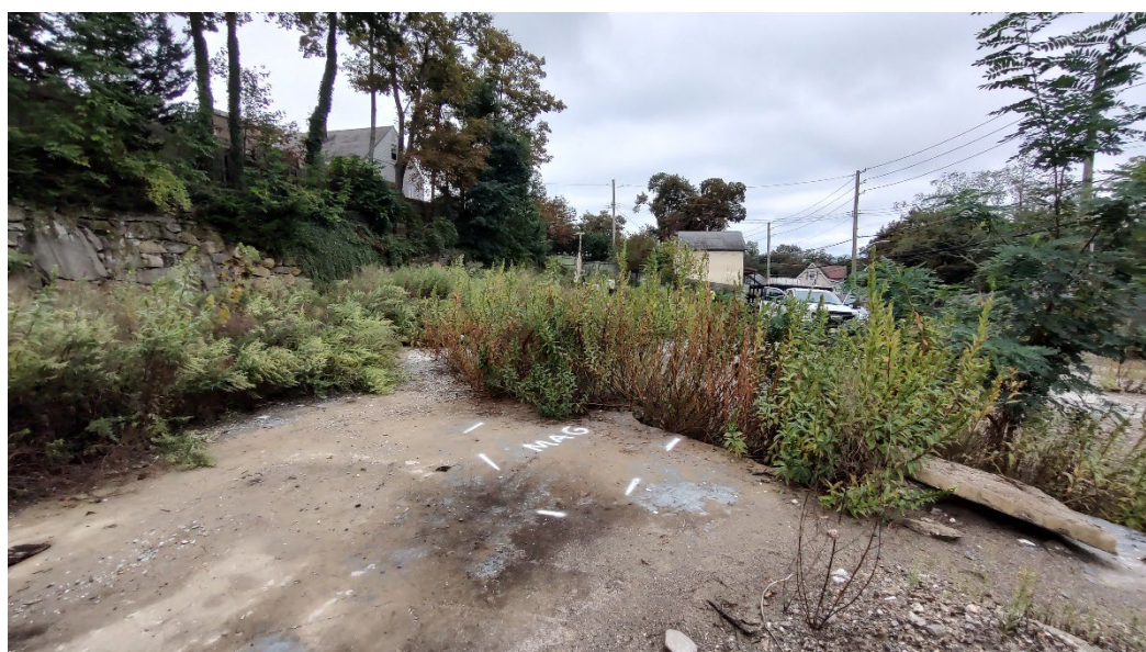
Photos 2 & 3– View of a magnetic anomaly on a raised concrete pad located along the east side of the site. This anomaly did not reveal any data during a GPR investigation of the area, though a second magnetic anomaly (shown below) was also detected within approximately 10 feet of each other.
