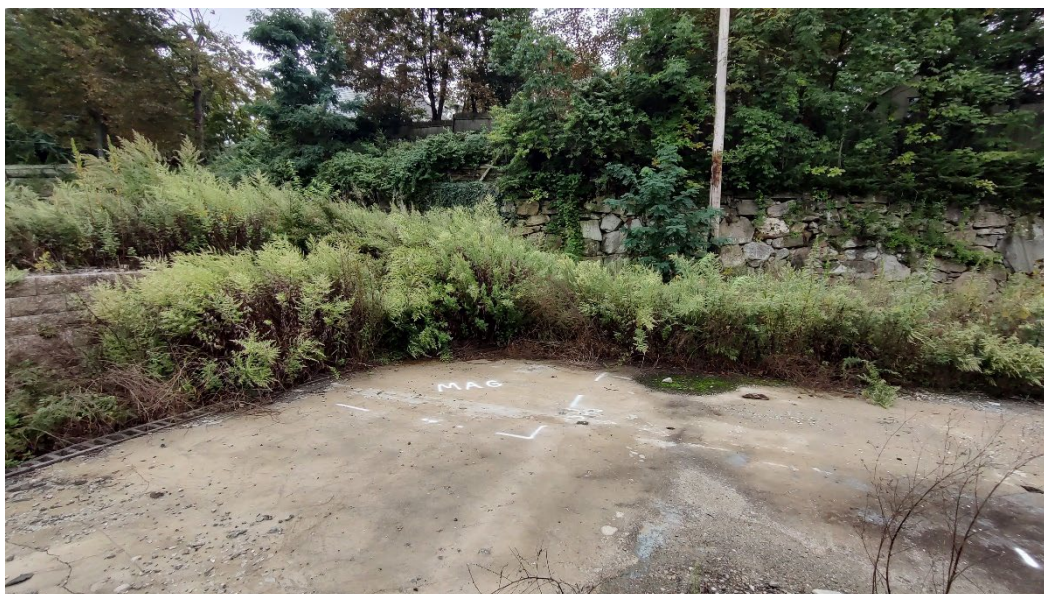
Photos 2 & 3– View of a magnetic anomaly on a raised concrete pad located along the east side of the site. This anomaly did not reveal any data during a GPR investigation of the area, though a second magnetic anomaly (shown below) was also detected within approximately 10 feet of each other.
