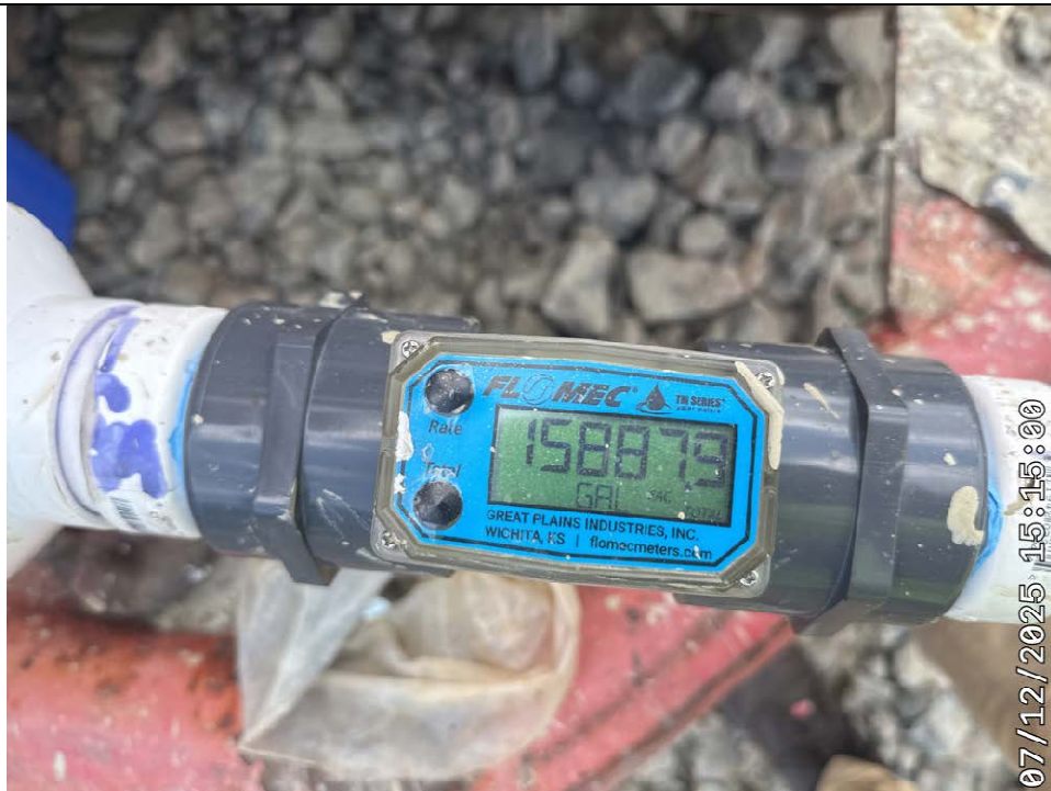
Photo 4: Flow totalizer on dewatering system effluent piping.
