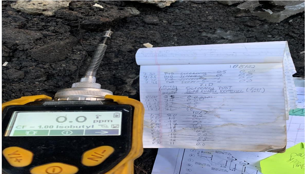
Photo 2 – PID screening of cleared slab area
