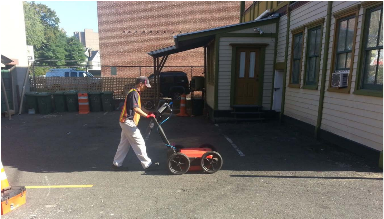
Geophysical survey to identify potential underground tanks (USTs).
