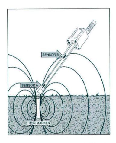
To perform a sweep, the locator is swept from side to side. When the locator comes within range of an iron object, the audio signal will peak, the bar graph will expand positive or negative, and the digital readout will peak as shown below; it is this peak response that indicates the existence of a metallic object buried underground.
