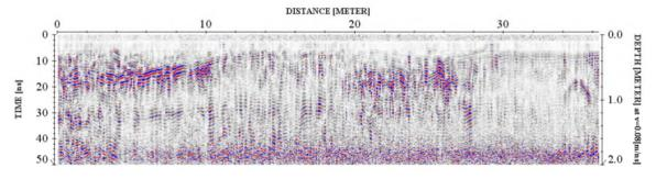
The above example shows the significance of data processing. The last image (step 5) has higher resolution than the starting image (raw data – step 1) and describes the subsurface anomalies more accurately.
