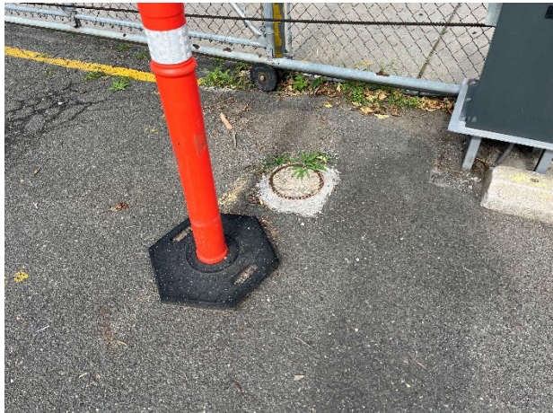
View of existing monitoring well MW-1 that is inaccessible and will need to be reinstalled.
