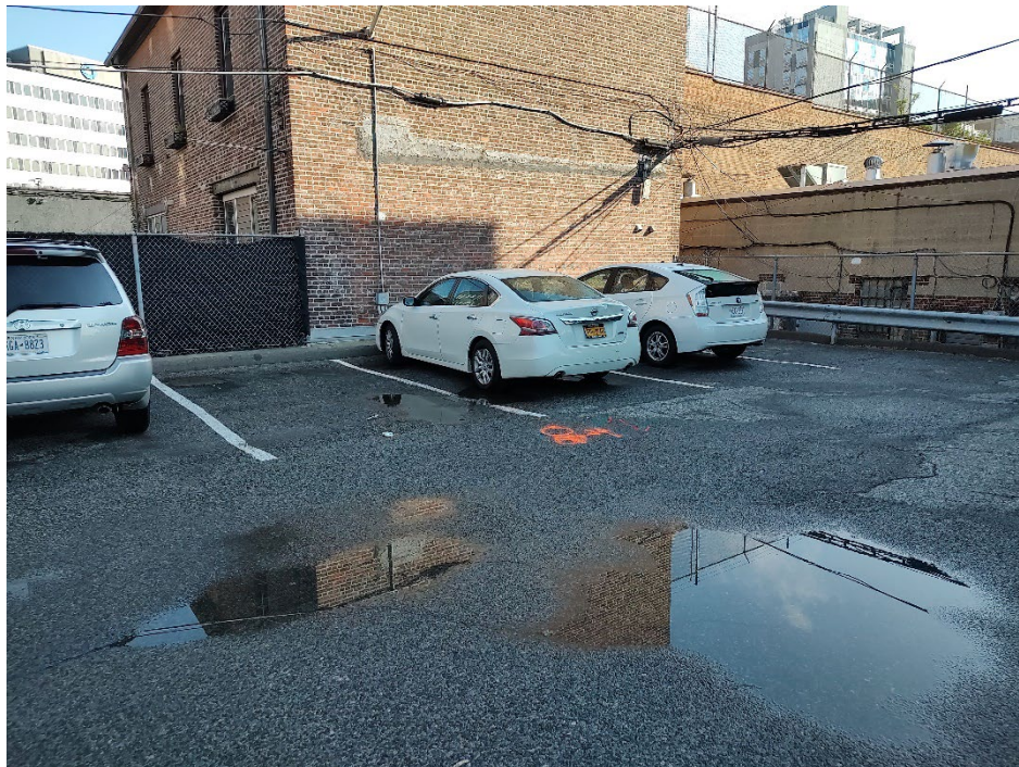
Photo 3 – Additional view of the electrical line powering one of the site lights in the lot (in front of the Nissan sedan). Due to the presence of this electrical line, Coastal suggested to shift the location of the soil boring (marked in orange).
