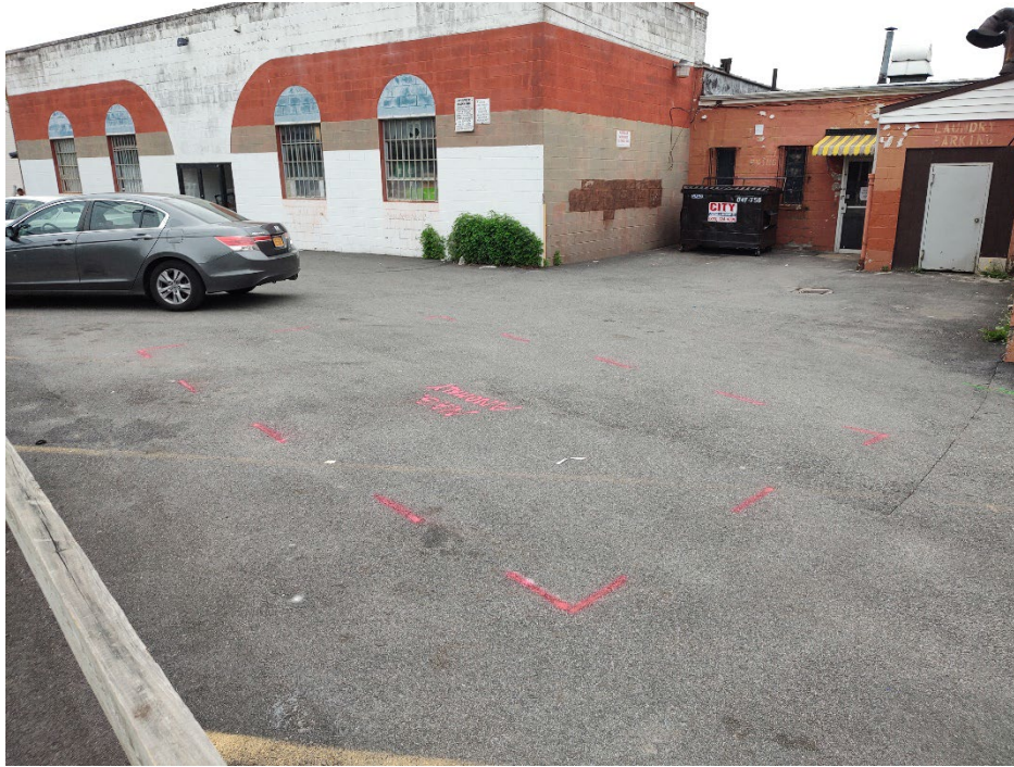
Photo 2 – View of the largest anomaly detected only with the TW-6 Magnetometer (not visible with GPR). This was positioned behind the laundromat at #154.
