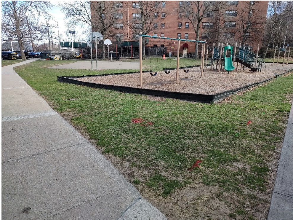
Photo 3 – View of the proposed soil boring locations within the area near the playground. A storm drain (marked in green) and electrical line (marked in red) were located here.
