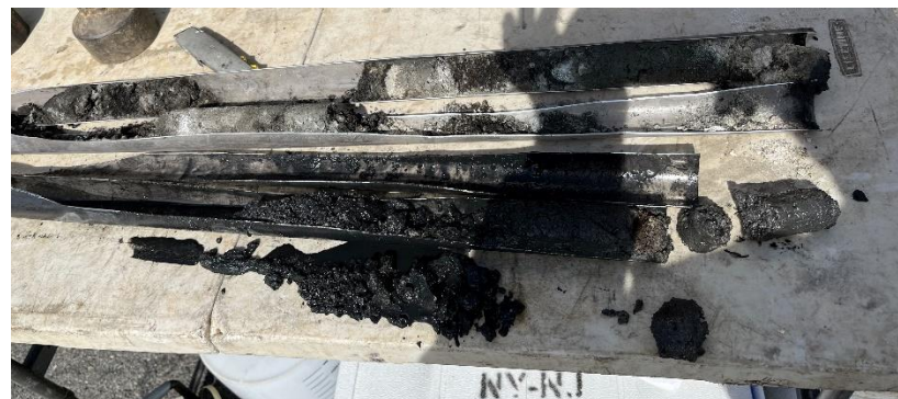
Photo 2 – Close up view of soil core at SB-11. Strong odor/PID reading, and discoloration were present at this location, among others.
