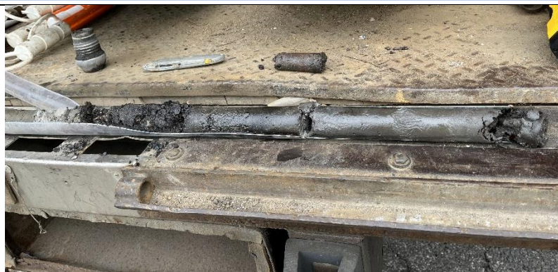
Photo 1 – Close up view of soil core at SB-9. PS&S field screened the soil cores using a PID meter and collected a grab (VOC) sample at the depth corresponding with the highest reading. Composite samples were collected across the entire soil core.
