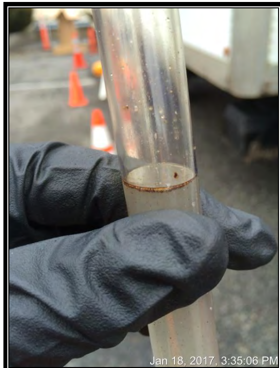
Photograph showing free-product in groundwater from GB-3 TW
