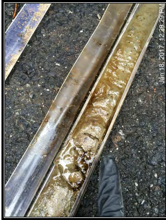
Photograph showing free-product in macro-core sample from GB-2 (8-12 ftbg)
