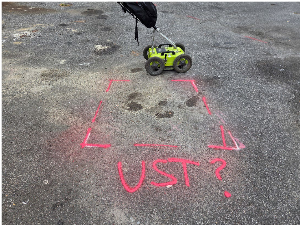
Photos 8 & 9 – Views of the areas investigated for suspected subsurface anomalies. The photo above shows the locations of two known USTs (white markings and arrow), while the subsurface detection below (marked in pink) was measured to be a square of approximately 3'x3' and not likely to be a UST. The additional area indicated by the arrow was investigated but no significant subsurface detections were found.
