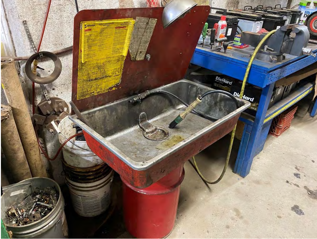
P.23 Auto Repair Shop – Parts Washer
