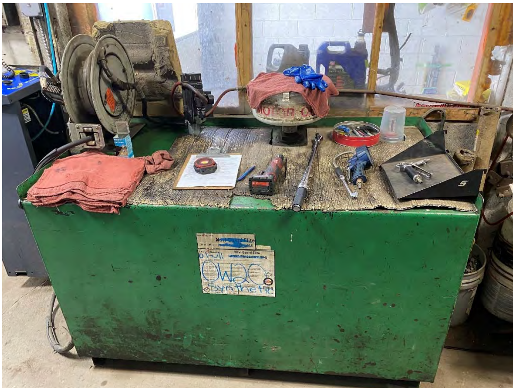
P.24 Auto Repair Shop – Motor Oil AST
