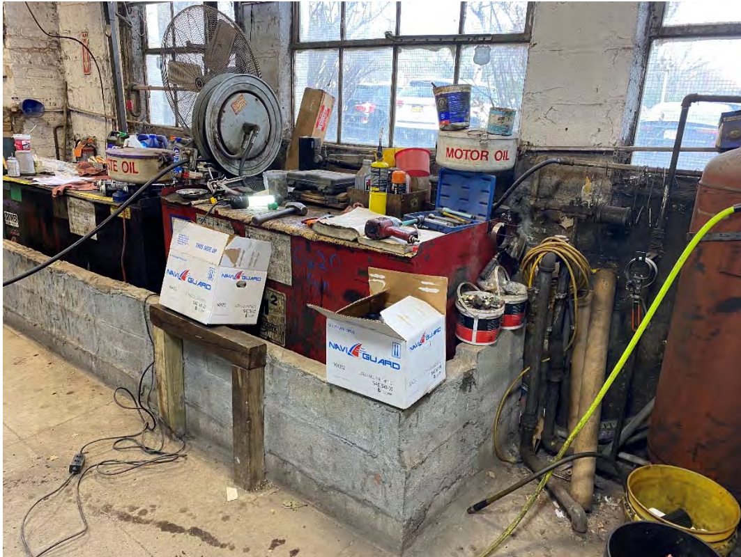
P.27 Auto Repair Shop - Waste Oil ASTs and Containment
