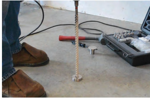
Figure 4. Using the Drilling Guide.
