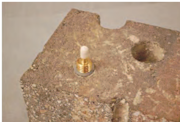
Figure 4. Installed Vapor Pin™.
