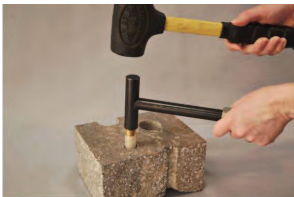
Figure 2. Installing the Vapor Pin™.
