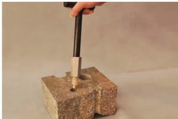
Figure 8. Extracted Vapor Pin™.
