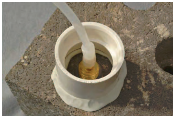
Figure 6. Water dam used for leak detection.
