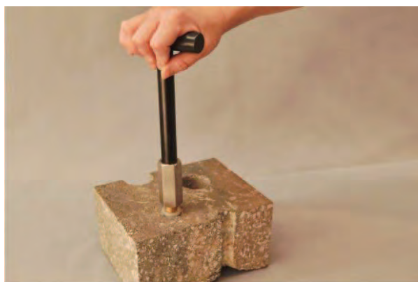
Figure 7. Removing the Vapor Pin™.
