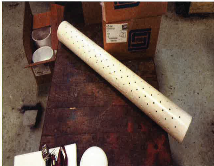
Photograph 4: View of one of the 4-inch diameter PVC perforated pipe with eight (8) rows of 32 holes (totaling 256 holes) drilled to allow air flow from the sub-slab materials in the EEA. A similar PVC perforated pipe was situated in the WEA.
