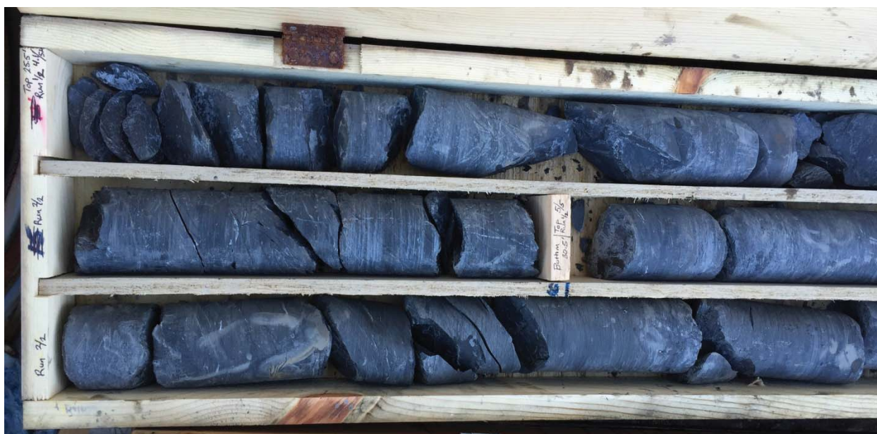
Photograph 12: Bedrock core of MW-10D starting at 25.5' below ground surface in top left of photograph.
