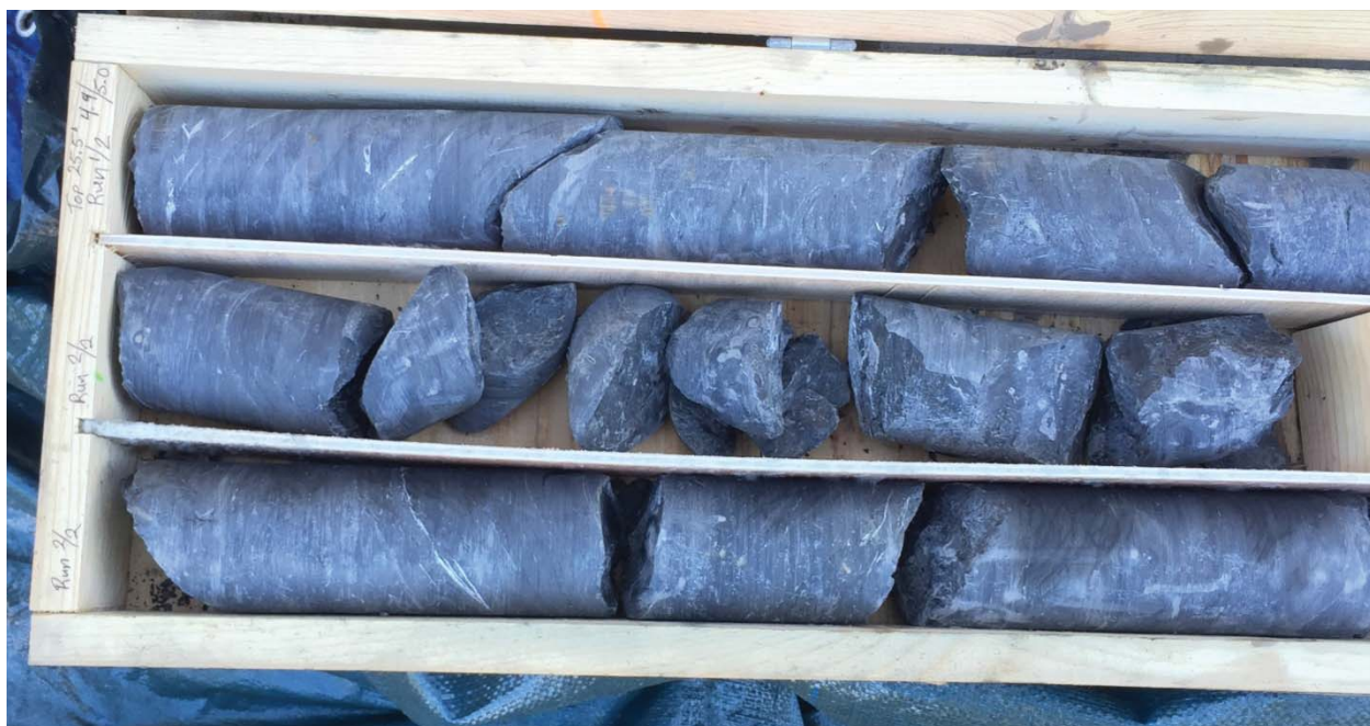
Photograph 9: Bedrock core of MW-7D starting at 25.5' below ground surface in top left of photograph.
