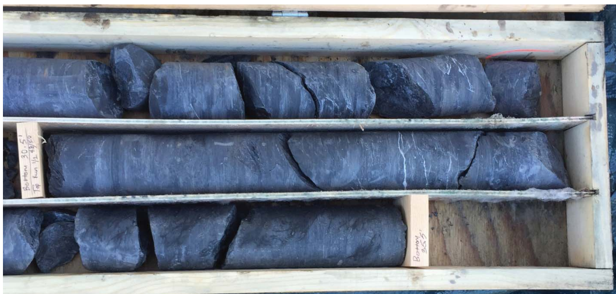
Photograph 10: Bedrock core of MW-7D ending at 35.5' below ground surface in top left of photograph.
