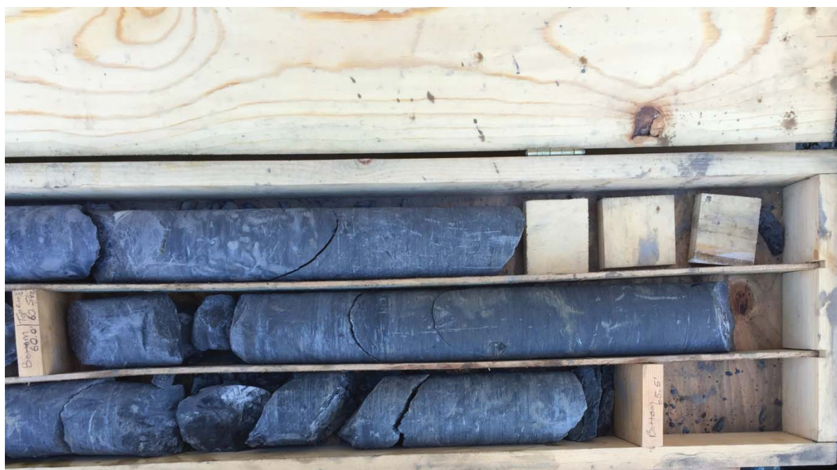
Photograph 2: Bedrock core of MW-6D' ending at 65.5' below ground surface in bottom right of photograph.
