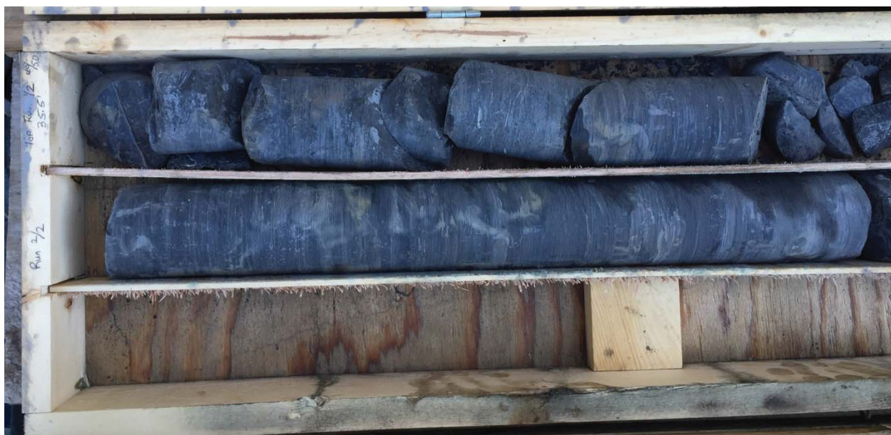
Photograph 14: Bedrock core of MW-10D at 35.5' – 40.5' below ground surface.
