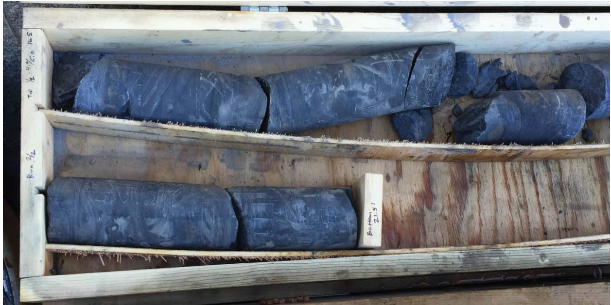
Photograph 7: Bedrock core of MW-7S starting at 16.5' below ground surface in top left of the photograph. End of bedrock core is also shown at 21.5' below ground surface.
