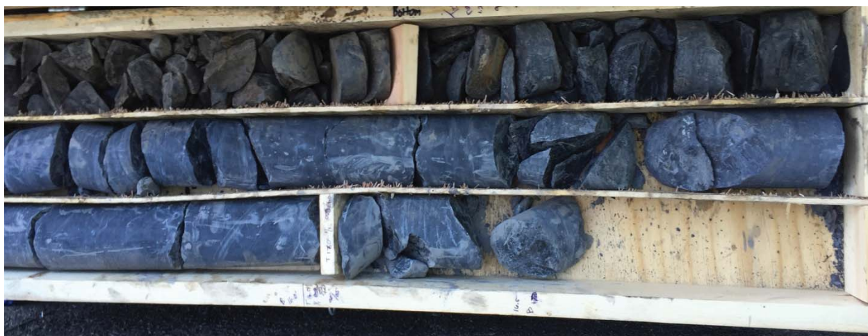
Photograph 6: Bedrock core of MW-7S ending at 16.5' below ground surface in bottom of photograph.
