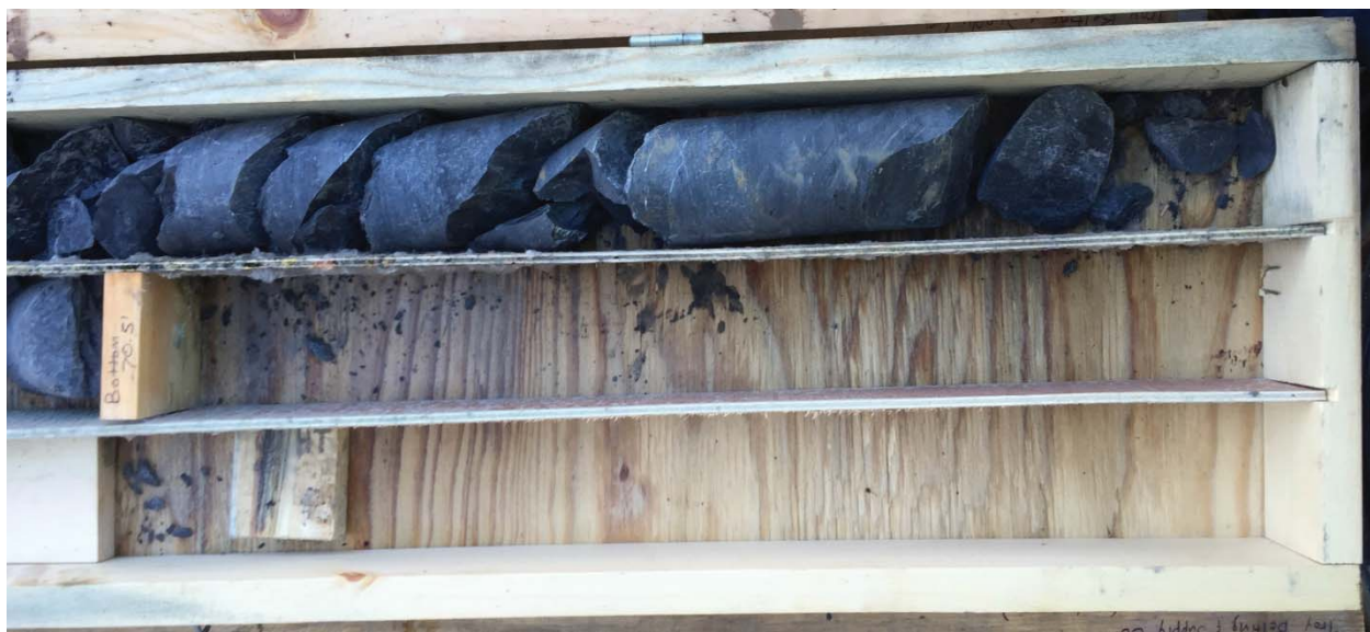
Photograph 4: Bedrock core of MW-6D' ending at 70.5' below ground surface in middle left of photograph.
