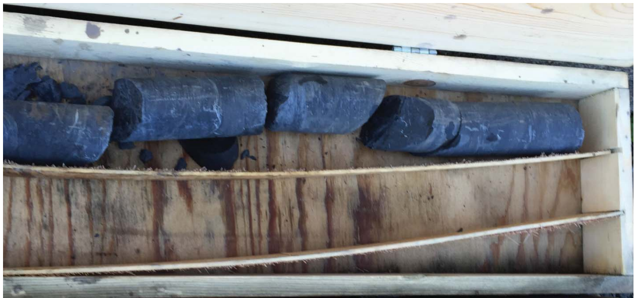
Photograph 8: Bedrock core of MW-7S at 17.0'-19.0' below ground surface.
