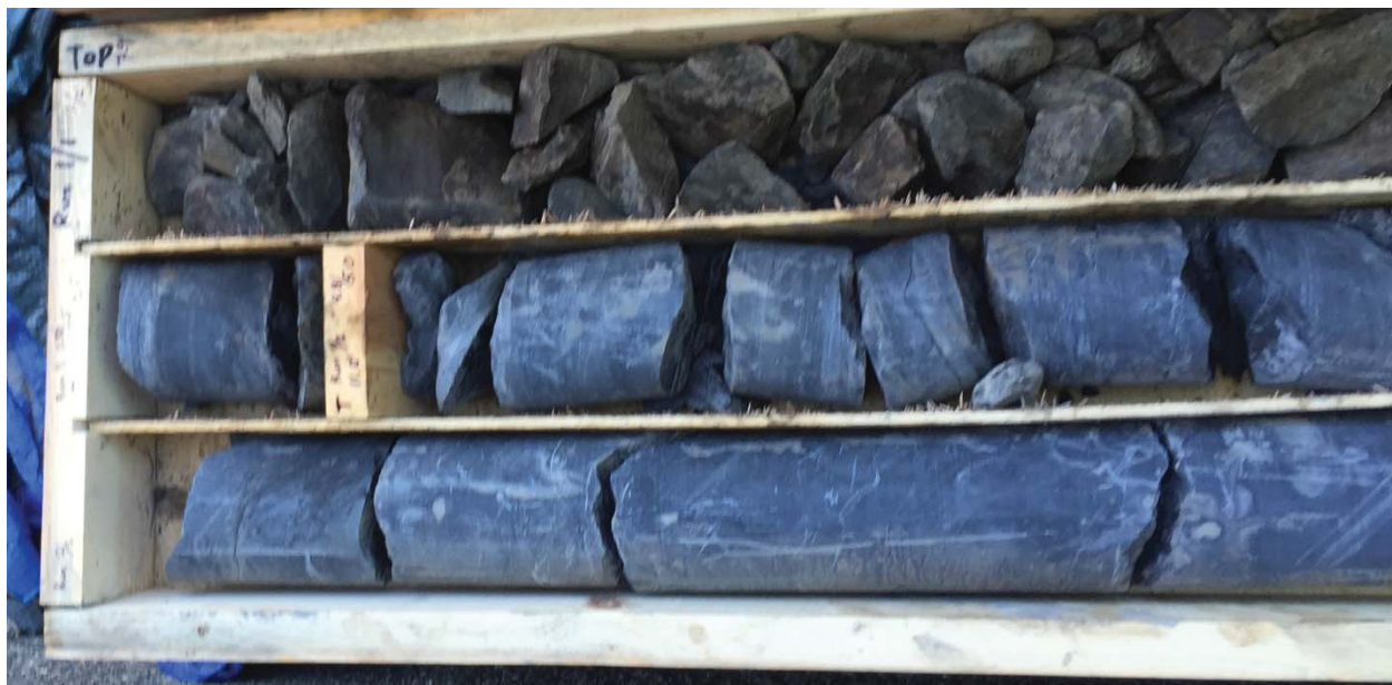
Photograph 5: Bedrock core of MW-7S starting at 6.0' below ground surface in top left of the photograph.
