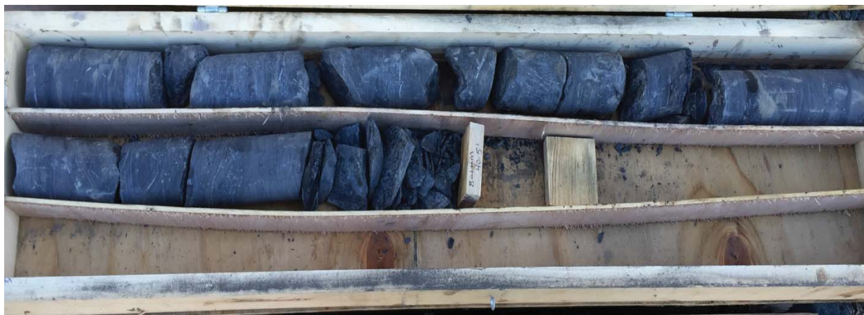
Photograph 11: Bedrock core of MW-7D at 35.5' – 40.5' below ground surface.
