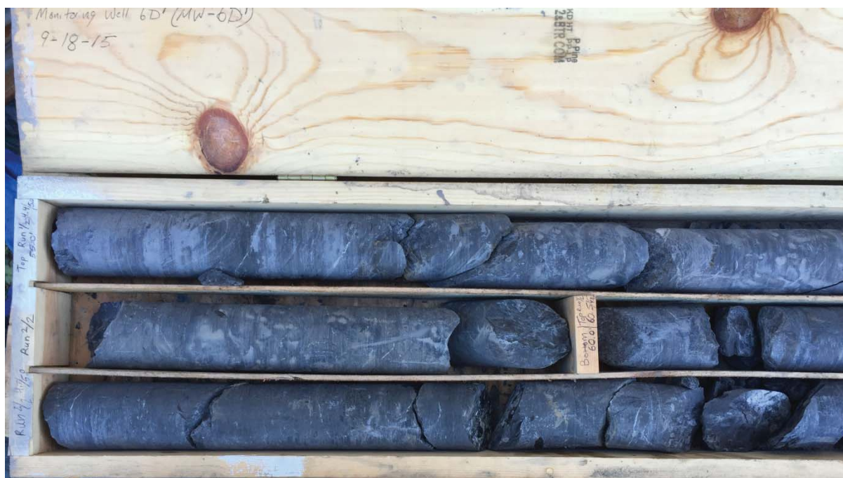
Photograph 1: Bedrock core of MW-6D' starting at 55.0' below ground surface in top left of photograph.
