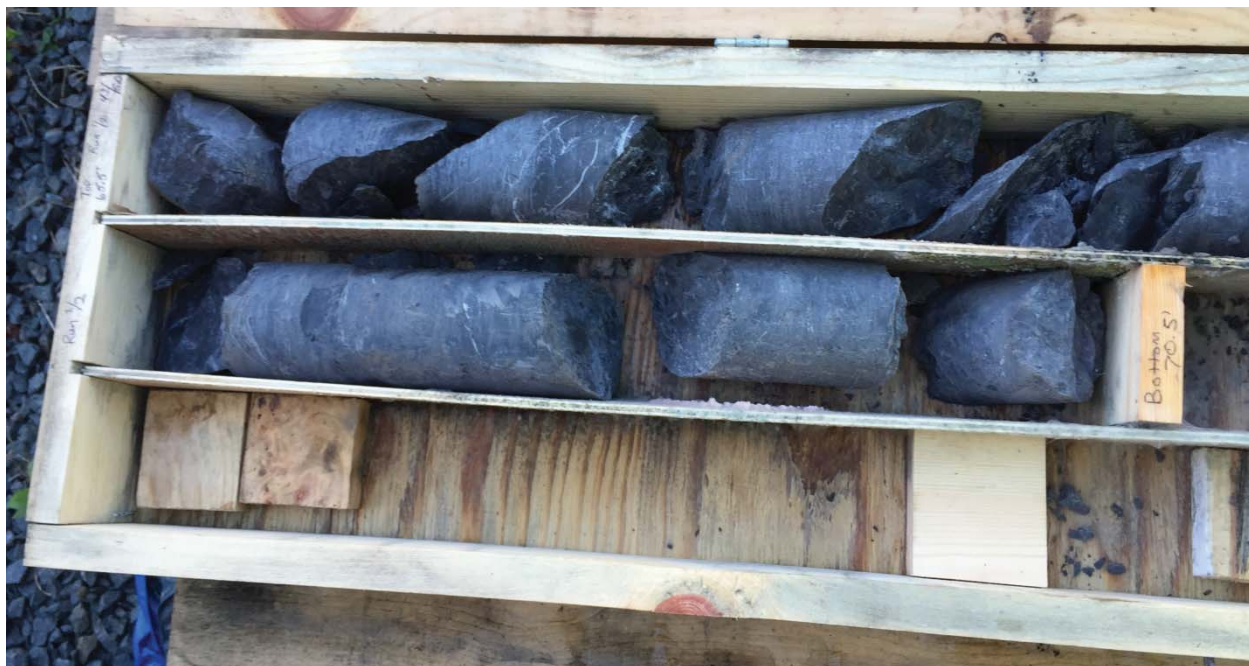
Photograph 3: Bedrock core of MW-6D' starting at 65.5' below ground surface in top left of photograph. Bottom of core also present at 70.5' below ground surface.
