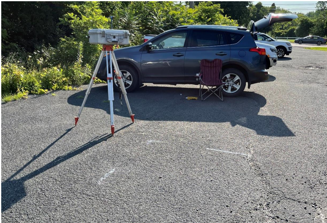
Photograph 5: Representative photograph of perimeter air monitoring equipment used throughout IRM construction during ground intrusive activities. View looking east. (Photo taken 7/23/21).
