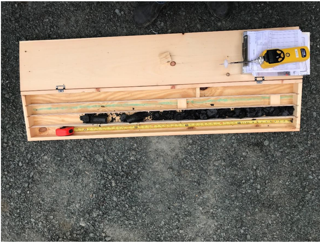
Photograph 35: Collected 5-foot rock core of shale bedrock. (Photo taken 10/8/21).
